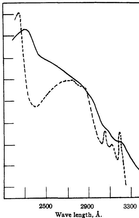
Fig. 2b.—Absorption spectra: ———, phenyl-di-(2-naphthyl)-carbinol (solvent dioxane); - - - - -, calcd. summation curve for 2 moles of 2-methylnaphthalene and 1 mole of toluene.
